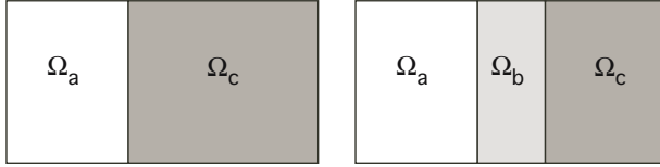
Fig. 1. Non-overlapping (left) and overlapping (right) coupling of atomistic and continuum models
